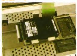
Put the drive and cradle back into the computer, with the cable facing to the left and the highest Lshaped part of the cradle to the rear. Once the case is put back together, these will hold the cradle steady against the case.
